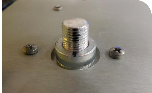
Figure 8. Rotate Shutter Adjustment Screw Clockwise
