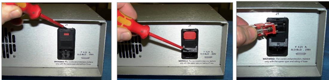
Figure 10. Replacing Fuses in the Power Supply
