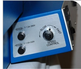
Figure 21. Conveyor Control Panel, Side
