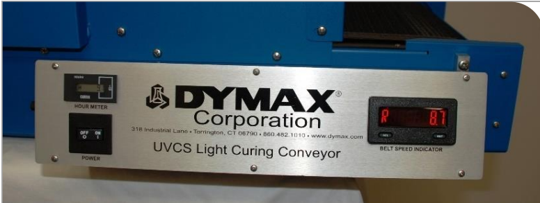
Figure 20. Conveyor Control Panel, Front
