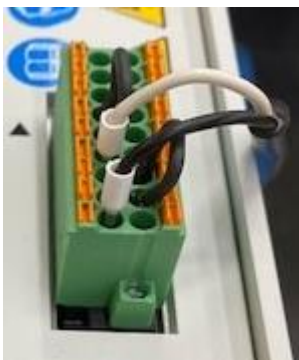
Figure 16. LED On/Off Pins 6 and A Installed with jumpers.
