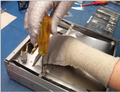
Figure 30. Tighten the M4 x 6 mm End Screws
