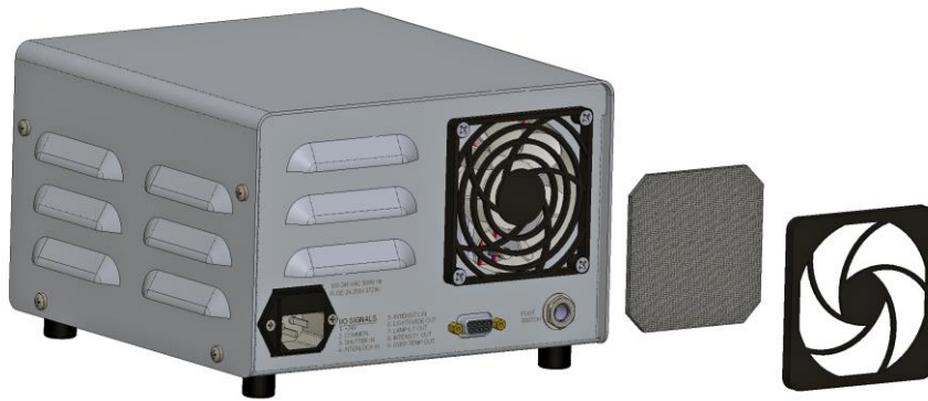
Figure 10. Cooling Fan Filter & Cover
